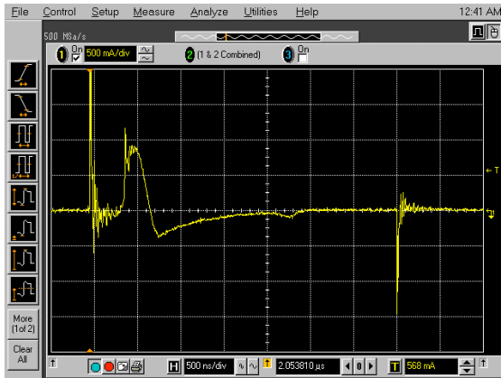
Figure 9. Secondary discharge recorded at different laboratory showing delayed negative pulse. Scale factors: 500 mA/div and 500 ns/div.
