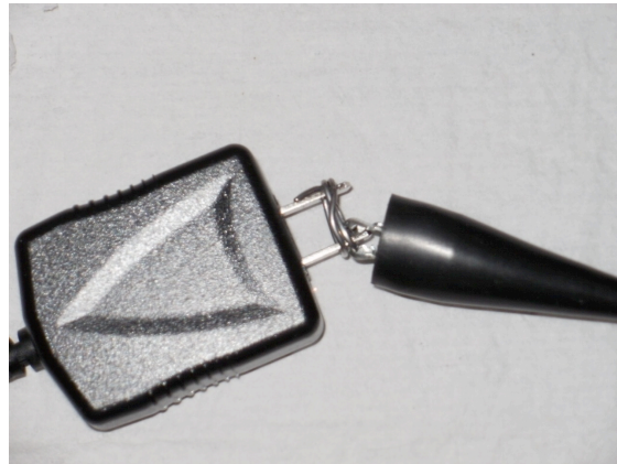
Figure 2. Shorting of the mains connections.
