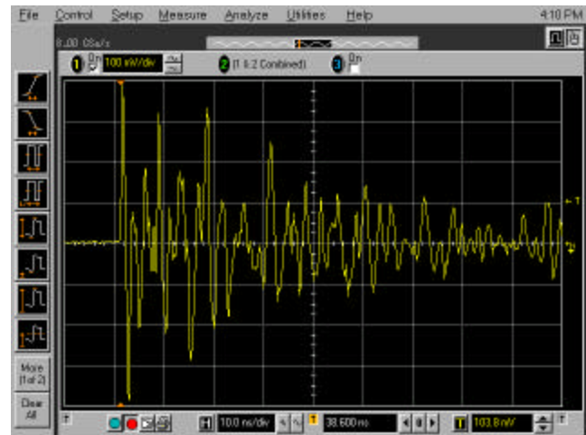
Figure 9: Radiated Field, Equipment Maintenance The low ringing frequency in Figure 10, between 15 and 20 MHz was likely due to the source involving a large structure. The observed frequency was the natural resonant frequency of that structure. One wavelength in free space at 15 MHz is 20 meters so the structure might be comparable to a significant fraction of that size. Possibly a whole bank of racks was involved. One of our authors has personally observed a similar case where such an event caused interference with optical transmission circuits within a large equipment installation.
