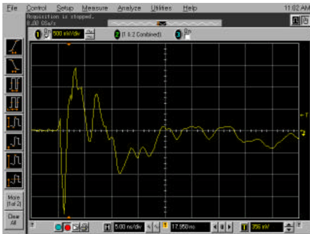
Figure 2: Radiated Field, +500 Volt Cable Shield Discharge
