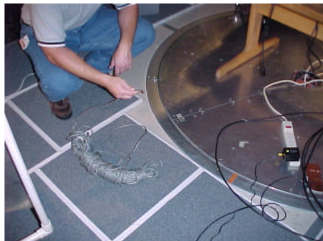
Figure 3a: Bundled Unshielded Cable Used in Discharge
