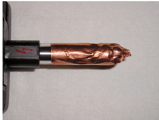
Figure 2. High pass filter on ESD simulator.
