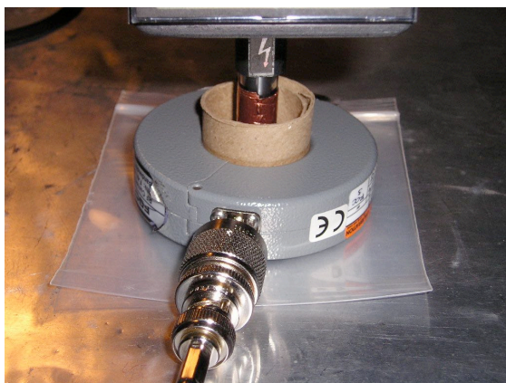
Figure 3. Measuring the filtered discharge current.
