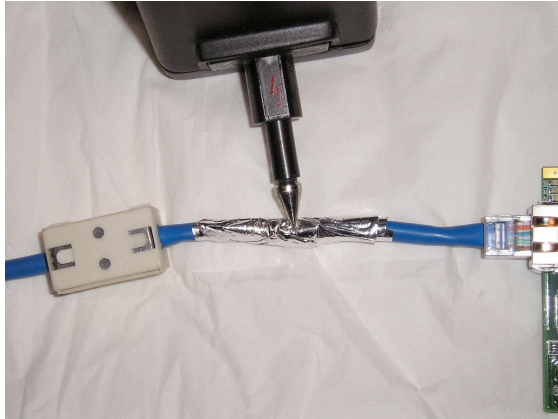
Figure 5. Injecting ESD energy into a cable.
