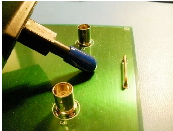
Figure 1. Coupling ESD energy to a PCB.
